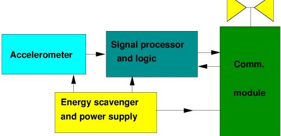
The operation of each node is based on energy scavenged from vibrations and the local processing of the information from an accelerometer
