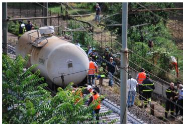
Derailment of a freight car may remain unnoticed for several kilometers, if it is far from the locomotive, and severe damage to the infrastructure can result
