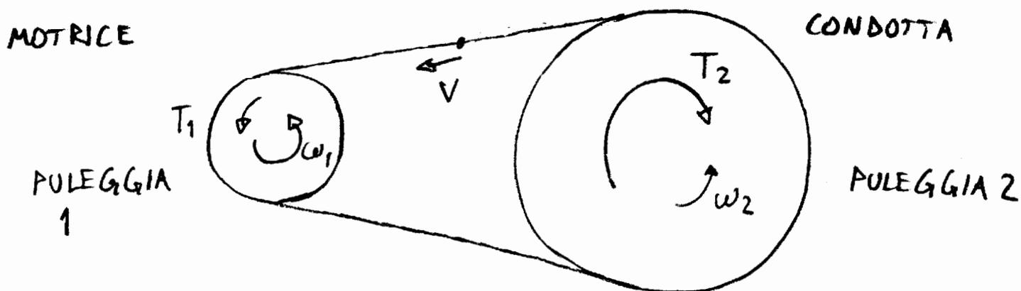
→ A DIFFERENZA DELLE RUOTE DENTATE  $\omega_1$  E  $\omega_2$
